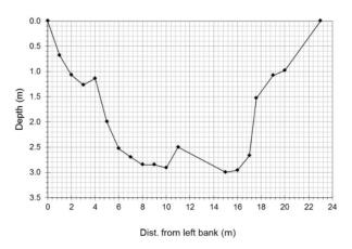
6. Have students calculate the stream discharge by multiplying the velocity times the crosssectional area. Result will be in m<sup>3</sup>/sec. Can have students convert to ft<sup>3</sup>/sec (cfs) to match USGS data by multiplying result by conversion factor of 35.3 ft<sup>3</sup>/m<sup>3</sup> (1 m<sup>3</sup> = 35.3 ft<sup>3</sup>).
